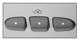
HomeLink, a combined universal transmitter and receiver, provides a convenient way to replace up to three hand-held transmitters used to activate devices such as gate operators, garage door openers, entry door locks, security systems and home lighting. Additional HomeLink information can be found on the internet at www.homelink.com or by calling 1-800-355-3515.
